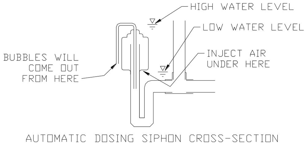
3.5.4. Using a piece of hose or small diameter pipe and a squeeze bulb (or some other method) bubble air under the bell until it is full of air and you see it begin to bubble up inside the dosing compartment from underneath the bell.
